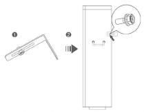
2) Make the back side of the battery close to the wall, and then mark locations of two assembly holes. Drill two holes and secure the battery to the wall in the same way as mentioned above in 4.3.1.
